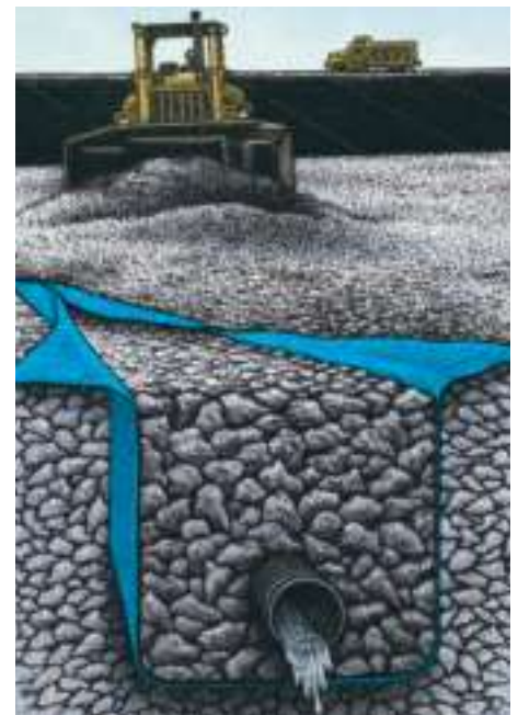
Propex woven monofilament geotextiles are very resistant to biological clogging, making them ideal for landfill leachate collection systems.
